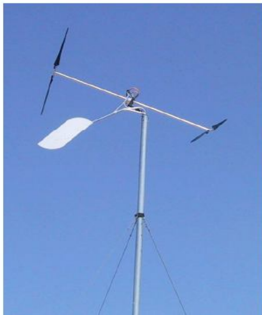
Co-axial, multi-rotor horizontal axis wind turbines
